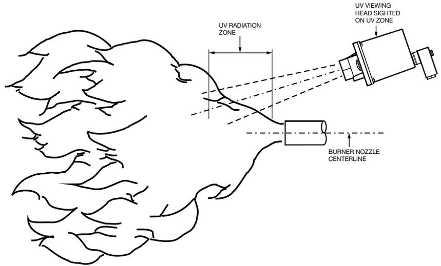
Example of sighting for Ultraviolet flame radiation (UV), or Infrared radiation (IR).
