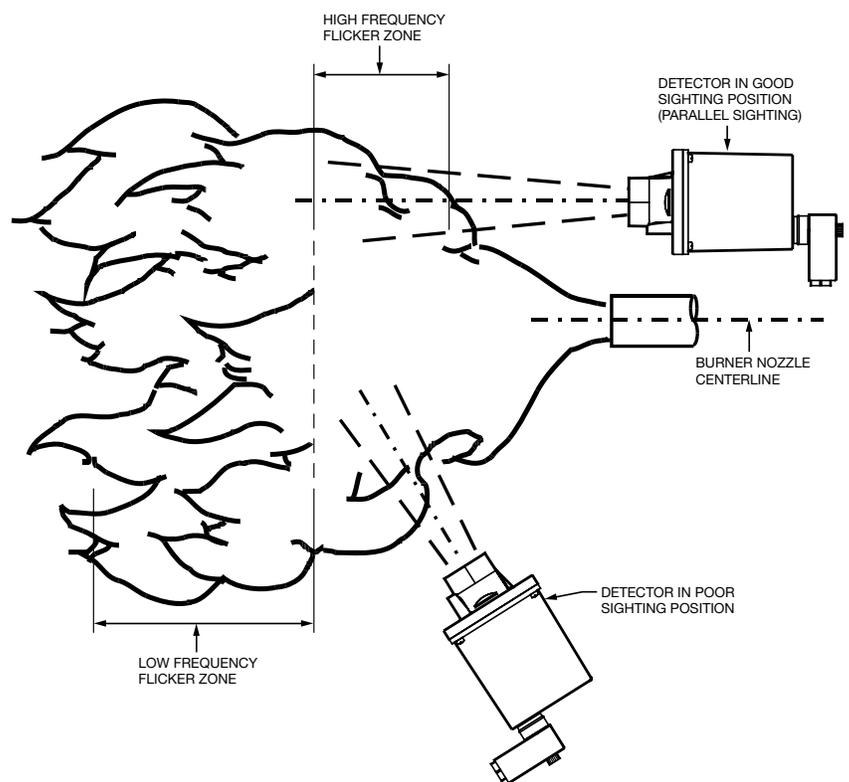
Example of sighting for Ultraviolet flame radiation (UV), or Infrared radiation (IR).
