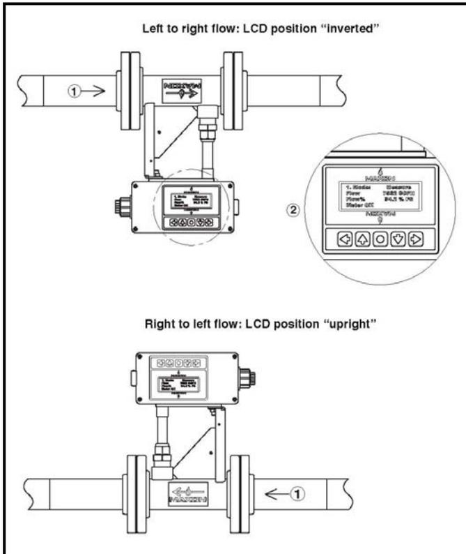
3.1.3. Flow sensor insertion: If the flow sensor assembly is provided separately or removed during flow body installation, the following procedure should be followed when re-inserting the sensor into the flow body:
